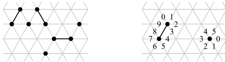
■ Figure 1 Left: Expanded and contracted particles. Right: particles with edge numbering.
