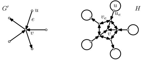
■ **Figure 3** The modification applied to a planar directed graph  $G'$ . The modification of Kaplan and Nussbaum does not include the original vertices inside of the new cycles. We need this since all the original vertices except a fixed source are targets in our algorithm.
